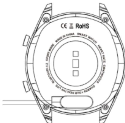
\*Be aware that the two contacts of the USB cable are not allowed to contact the conductor at the same time, or it will cause the circuit to burn.
